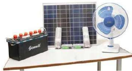
Fig 6. - Solar Lighting Systems
